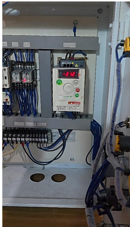
Figure 4. Initial Testing of Reverse Rotation Configuration
