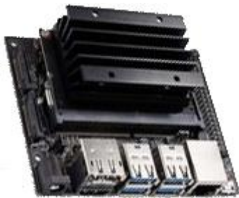
Gambar 4. Jetson Nano Developer Kit
