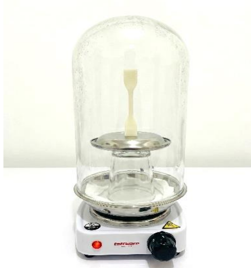
Figure 2. Acetone Vapor Smoothing Process
