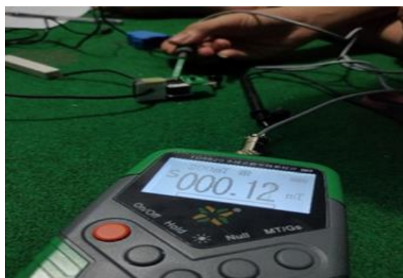
Figure 10. Magnetic Field Measurement Results Using a Gauss Meter Using 500 Turns
