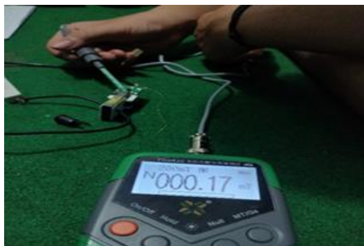
Figure 9. Results of magnetic field measurements using a gauss meter using 1000 turns
