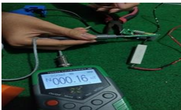
Figure 7. Magnetic Field Measurement Results Using a Gauss Meter Using 2000 Windings
