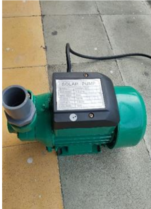
Figure 5. DC Water Pump
